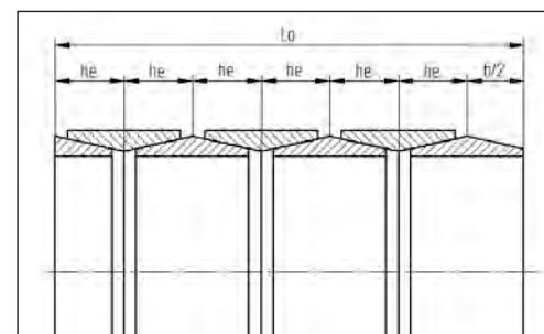
Fig. 8: Friction spring with 6 elements, ends 1 IR + 1 HIR
