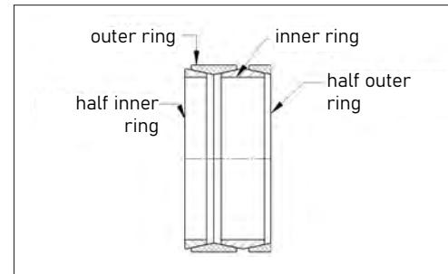
Fig. 6: Friction spring with HOR + HIR
